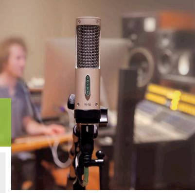
patented 2.5-micron offset ribbon element and rare earth Neodymium (Grade 52) magnets, the same one found in the rest of the R-Series mics, is made in-house at Royer HQ. The new custom transformer is USA-made, and the mic is hand-assembled at the company's Burbank factory. It comes with a 5-year warranty and the first re-ribboning is free. As a point of reference: I've had my R-121 for 17 years and it just got its first re-ribboning last year!
