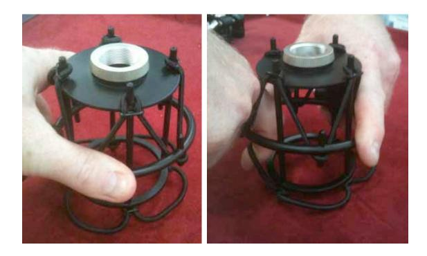
8. Pull hooked 2<sup>nd</sup> band through triangle and hook over shock ring post. Repeat with all 3 other sections of 2<sup>nd</sup> band. Adjust shock so that shock ring is parallel to table surface and tension is evenly distributed among band sections.
