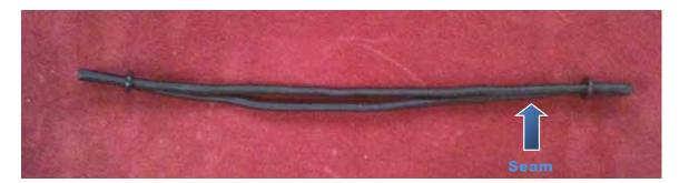
2. Fold band in half and roll 2 more small o-rings onto band about ½" from ends.
