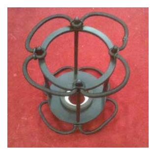
6. Turn carriage upside down and align outer shock ring over top of carriage. Maneuver shock ring and 1<sup>st</sup> band to hook band segments with all 4 posts of outer shock ring.
