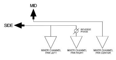
Figure 3 Typical M-S connection set-up
