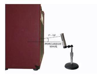
Slight off-axis positioning minimizes stressing the ribbon on loud sound sources.
