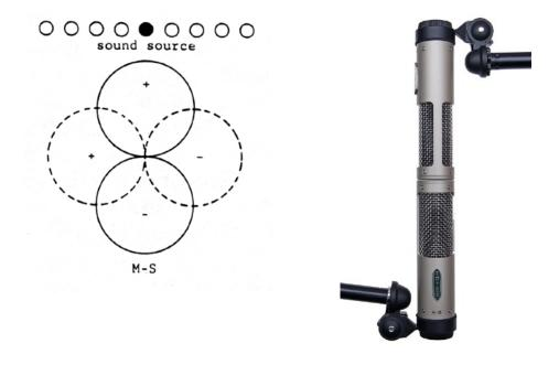
Figure 2 - Typical M-S Miking Technique
