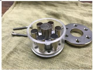
The design is such that most of the magnetic force is concentrated within the flux gap while minimizing stray leakage that could magnetize the EMT's steel reverberation plate.
