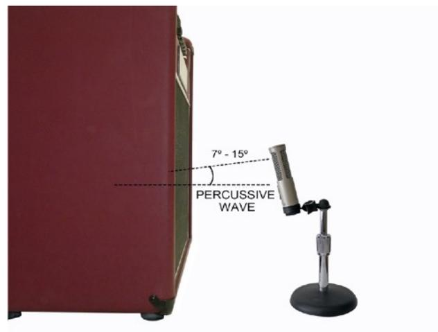
*Slight off-axis positioning minimizes stressing the ribbon on loud sound sources.*
