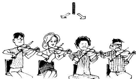
ambience. For violin, position the SF-24V horizontally, two or more feet above the instrument. For larger string sections, try placing the microphone slightly above the instrumentalists and angled down; a distance of three or four feet will do the job nicely.
